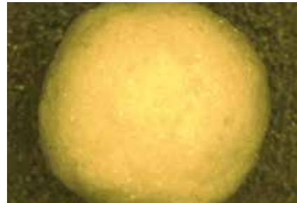
Figure 5: Single spherical lactose agglomerate (light microscope, magnification: 50x)
