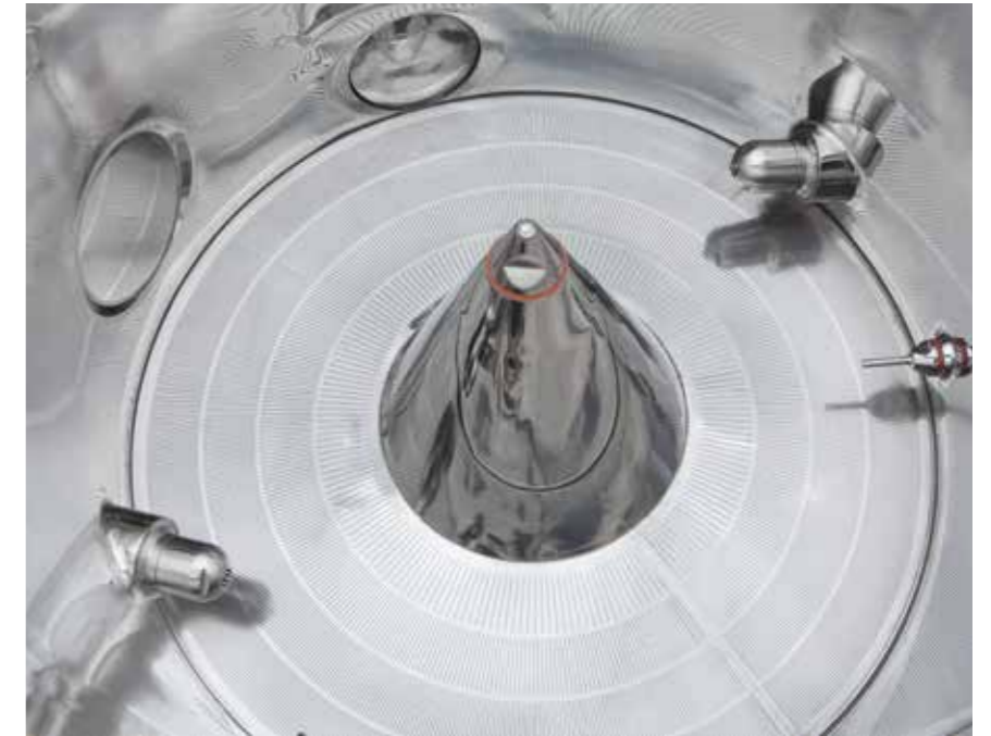
Figure 2: Bohle Uni Cone BUC® with tangentially mounted spray nozzles within a BFS 30
