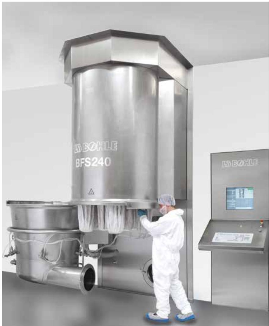
The L.B. Bohle product range of fluid bed systems contains machines from the BFS 3 in a laboratory scale up to the biggest type BFS 480. The Bohle Uni Cone BUC® optimizes the process.
