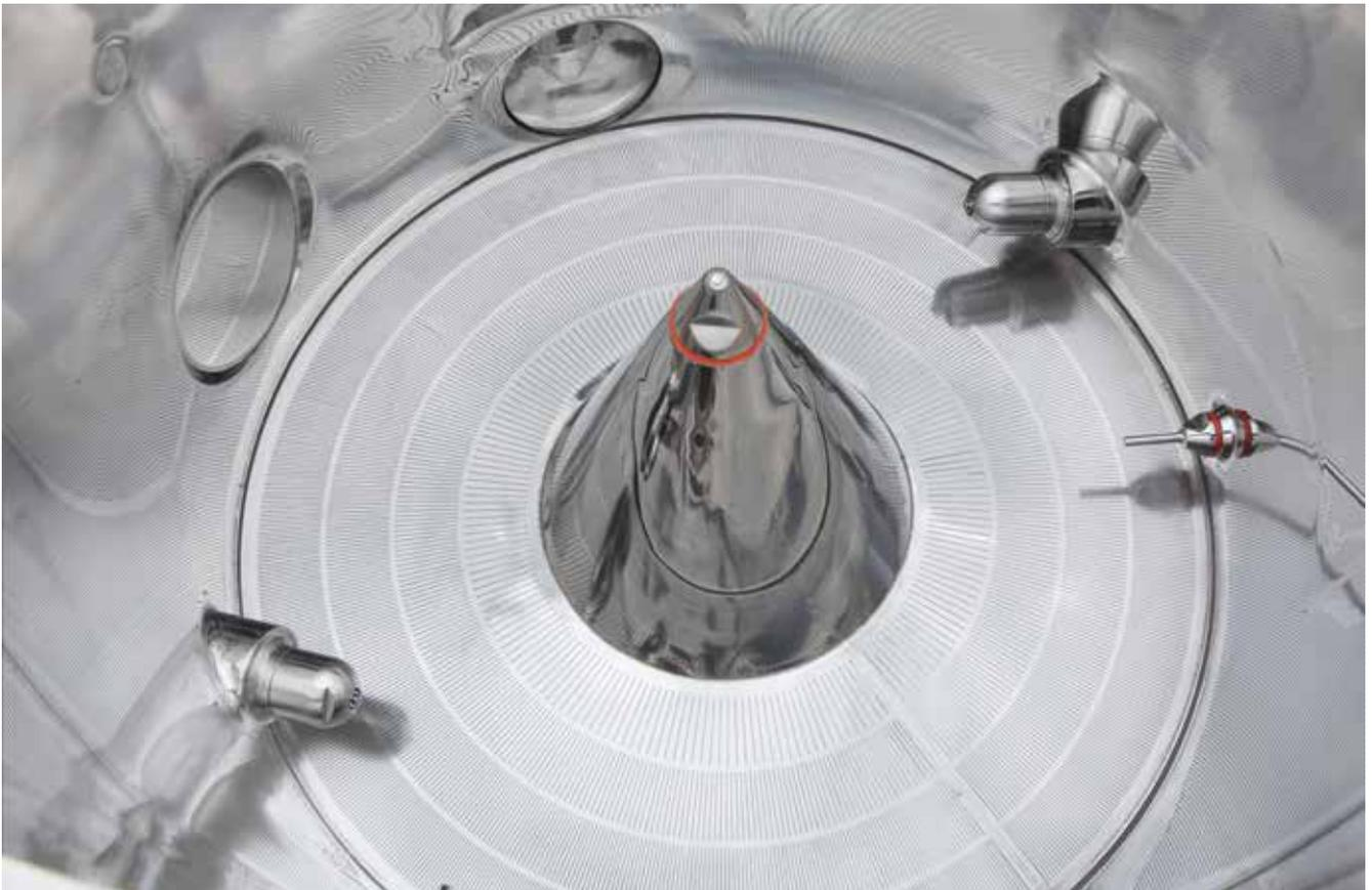
Bohle Uni Cone BUC® distributor plate with tangentially mounted spray nozzles.
